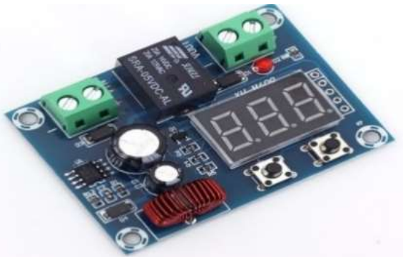
Gambar 2. 7 Low Voltage Disconnect
