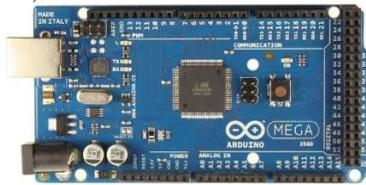
**Gambar 2. 1** Arduino mega 2560
