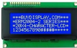
**Gambar 2. 3 LCD 20X4**
