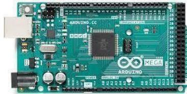
**Gambar 2. 5 Arduino Mega 2560**
