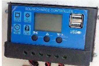
**Gambar 0.3 Solar Charge Controller**
