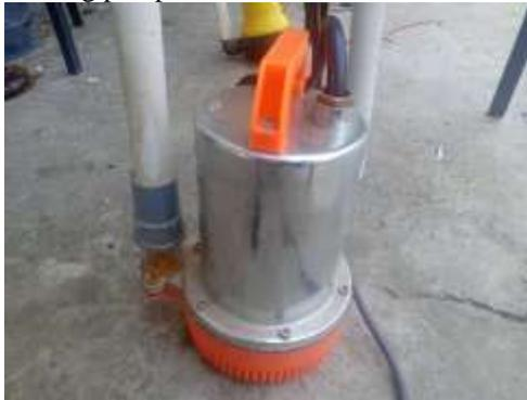
**Gambar 2.4 Pompa Submersible**
