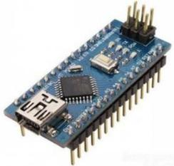
**Gambar 2.11 Arduino Nano** <sup>[23]</sup>
