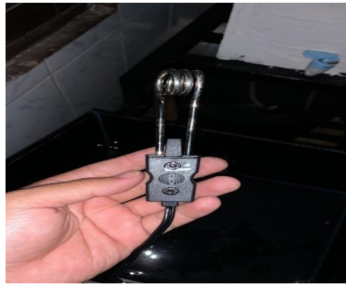
Gambar 2. 8 Water Heater Sumber : Peneliti, (2022)
