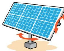
Gambar 2. 7 Panel Surya Dual Axis
