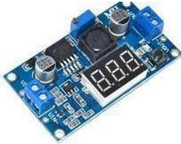
Gambar 2.9 Modul *Step Down Lm2596* <sup>[21]</sup>.
