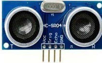
Gambar 2.2 Sensor Ultrasonik Hc – SR04<sup>[13]</sup>.
