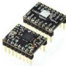
Gambar 2. 5 Driver motor A4988 [7]
