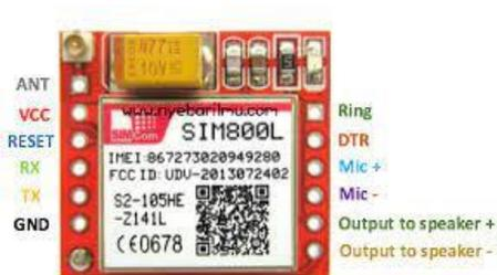
**Gambar 2.4 Modul GSM Sim 800L**
