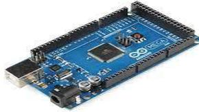
**Gambar 2.1 Arduino Mega2560**
