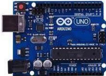
Gambar 2.1 Arduino Uno <sup>[5]</sup>
