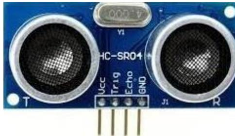
Gambar 2.9 Sensor Ultrasonik HC-SR04<sup>[13]</sup>
