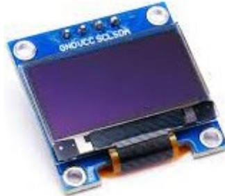
**Gambar 2.13** *OLED Display* 128 x 64
