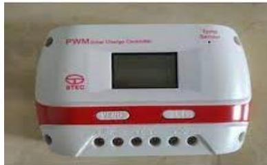
**Gambar 2. 2** *Solar Charge Controller*<sup>[11]</sup>.
