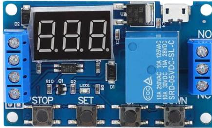
**Gambar 2. 15 Modul Relay Trigger Delay**
