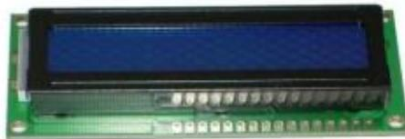
**Gambar 2. 9 LCD (*Liquid Crystal Display*)**
