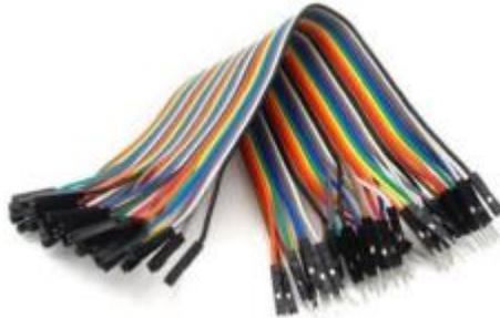
**Gambar 2. 13 Kabel Jumper**
