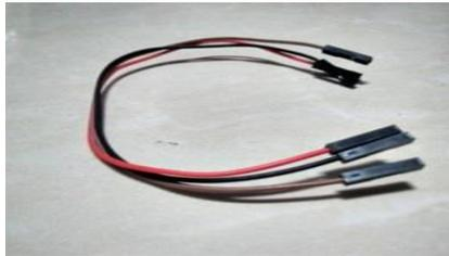
Gambar 2. 2 Kabel Jumper. [11]
