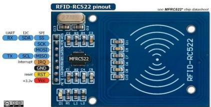
**Gambar 2.2** Modul RFID MFRC522
