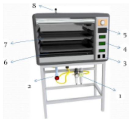
Gambar 2.4 Mesin tray dryer (Efrita et al., 2020)
