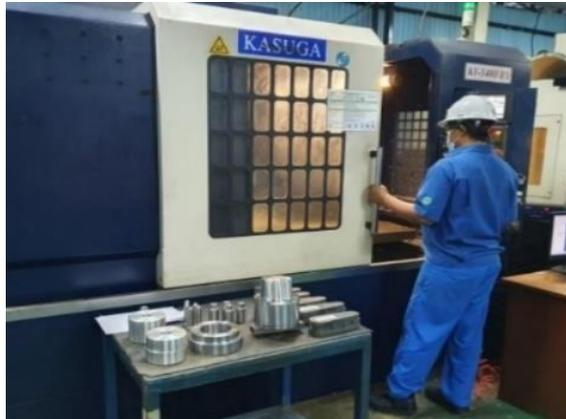
Gambar 2.5 Mesin CNC *milling*. (www.naratama.co.id)
