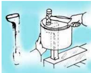
Gambar 2.3 Proses melipat tepian (Wirawan, 2008)
