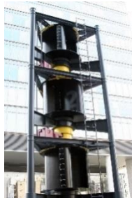
Gambar 2. 2 Turbin angin Sevonius [11]
