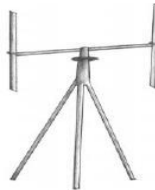
Gambar 2. 7 Turbin Angin Darrieus VAWT Tipe H-Rotor
