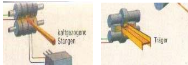
Gambar 2.4 Proses pengerolan (Widarto dkk, 2008)
