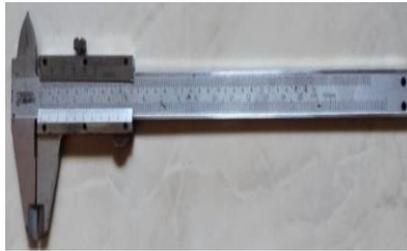
Gambar 2.6 Alat Pengukuran (Jangka sorong)
