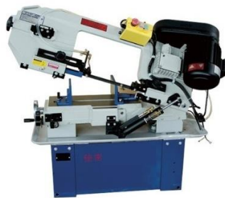
Gambar 2.16 Mesin gergaji pita (Majiid dkk, 2007)
