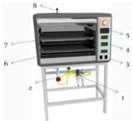
Gambar 2.5 Mesin tray dryer .
