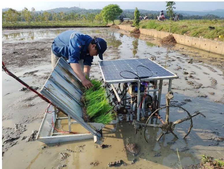
Gambar 4.43 Uji hasil mesin transplanter
