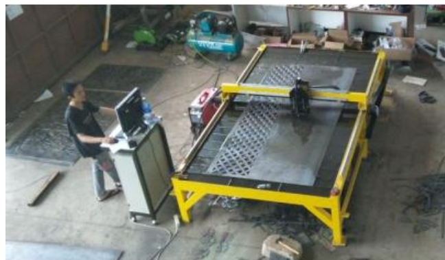
Gambar 2. 5 Mesin CNC plasma 3 sumbu (Rahman, 2019)
