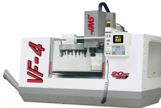
**Gambar 2.17** Mesin CNC *milling* (Act dkk, 2013)
