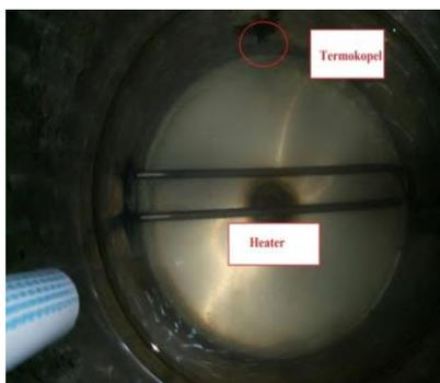
**Gambar 2.30** Termokopel dan *electric heater* (Sadad, 2016)
