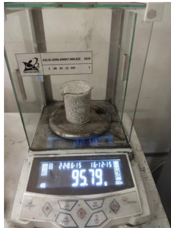
Penimbangan Biji Plastik PET Mesin “TIPIPIEL TWO”
