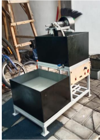
Gambar 7 Mesin oil skimmer tipe sabuk
