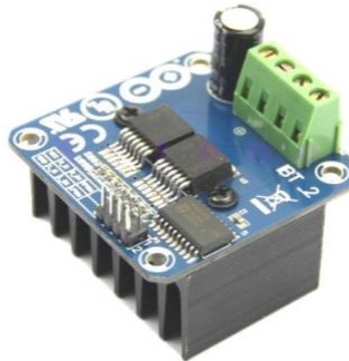
Gambar 2. 6 Motor Driver BTS 7960
