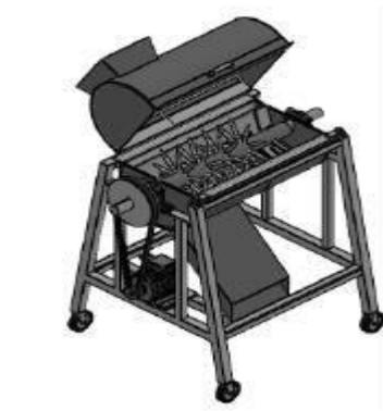
Gambar 2.2 Mesin Pengurai Sabut Kelapa (Satito dkk, 2020)
