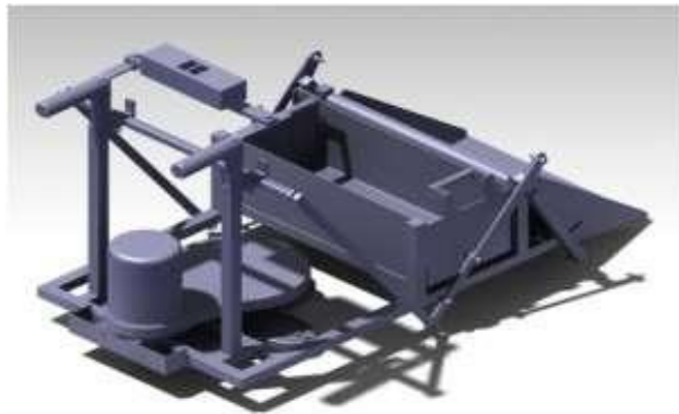
Gambar 2.1 Design and Modelling Cattle Shed Cleaning Machine (Shivakumar, 2015)
