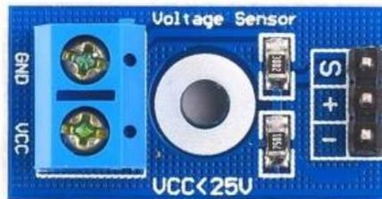
**Gambar 2. 8 Sensor Tegangan [24]**
