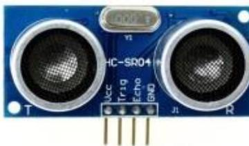
**Gambar 2. 14 Sensor Ultrasonic [30]**
