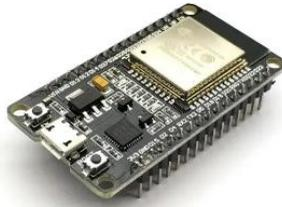
**Gambar 2. 4 NodeMcu ESP 32**
