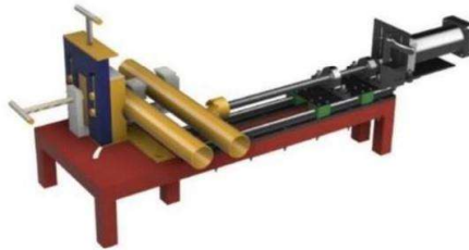
Gambar 2. 2 Rancang bangun mesin adjustable pipe notcher (Sumber : Assidiqi, dkk., 2021)
