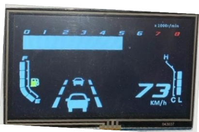
Gambar 4. 13 Tampilan RPM motor saat potensio 50%
