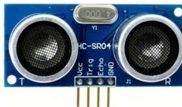
**Gambar 2. 5 Sensor *Ultrasonic***
