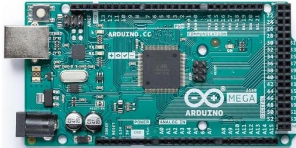
**Gambar 2. 3 Arduino Mega 2560<sup>[12]</sup>**
