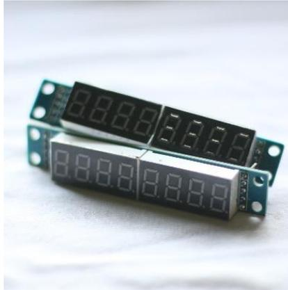
**Gambar 2. 9 Modul Seven Segment MAX7219**
