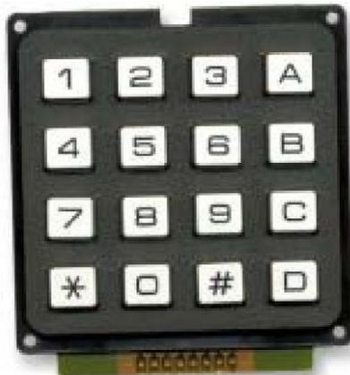
**Gambar 2. 11 Modul Keypad 4x4<sup>[21]</sup>**
