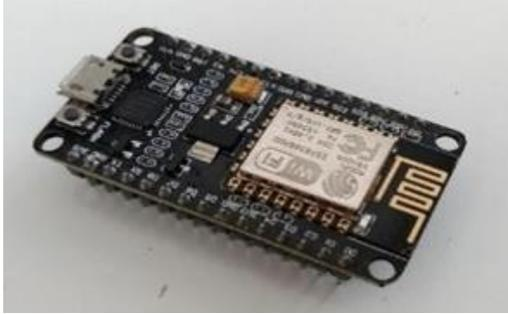
**Gambar 2.4** NodeMCU ESP8266
