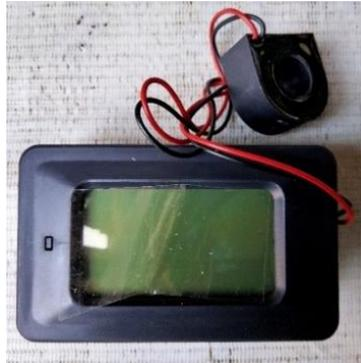
Gambar 2. 11 Wattermeter AC
