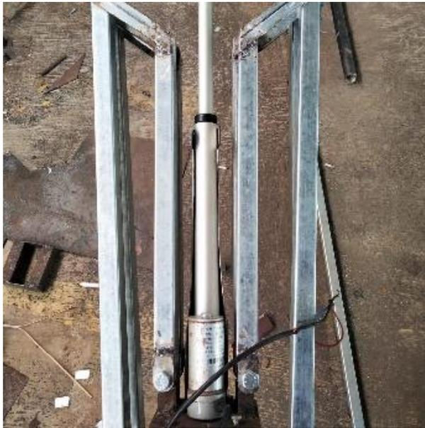
Gambar 2. 15 Motor Linear Aktuator
