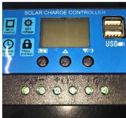
Gambar 2. 3 *Solar Charge Controller*
